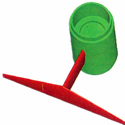
Fig. 9 Perspective view of the offset hydrofoil-cylinder part of the model shown in Fig. 8
