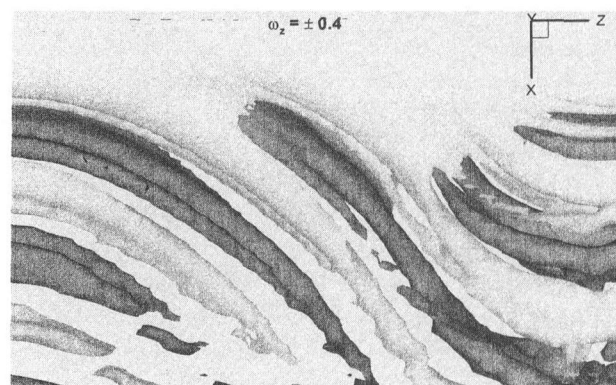
Fig. 14 Iso-surfaces of spanwise vorticity ( \omega_z = \pm 0.4 ) (with end plates) at time, t = 122.5 : no significant difference with the free-slip case (Fig. 7)
